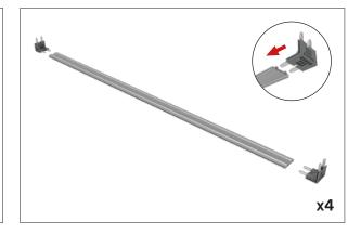
**Step 4:** Join the 2 vertical side frames to top and bottom horizontal frames.
