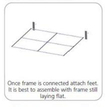
ALLEN KEY Use provided allen key, secure feet to bottom of frame by screwing bolt.
