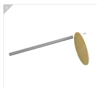
For proper pole alignment, begin by attaching poles to top shelf.
